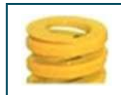
Extra Heavy load Max Deflection: 25% of Free length G-Series Color : Yellow
